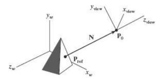
Specifying the view-plane normal vector N as the direction from a selected reference point  $P_{ref}$  to the viewing-coordinate origin  $P_0$ .
