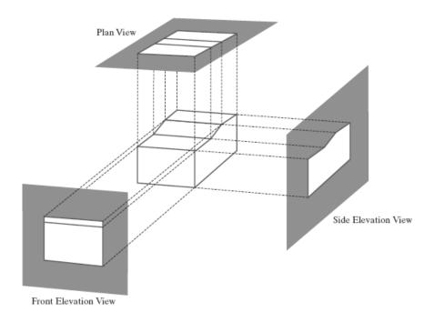
→ Front, side, and rear orthogonal projections of an object are called *elevations*; and a top orthogonal projection is called a *plan view*
